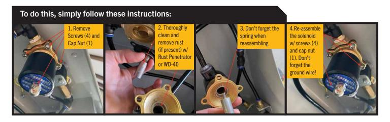
By taking the time to disassemble and clean the solenoid, you can help prolong the life and improve the performance of your MudMixer.
